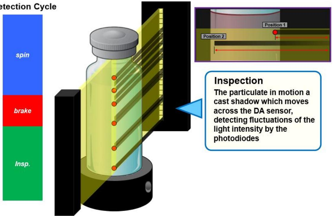
DIAGRAMMATIC REPRESENTATION OF DETECTION CYCLE OF LIGHT OBSCURATION PRINCIPLE IN AUTOMATED INSPECTION PROCESS
