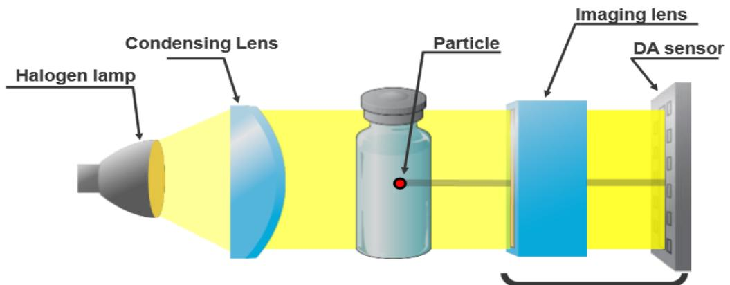
**The moving particles create a difference in light intensity while passing the (DA).**
