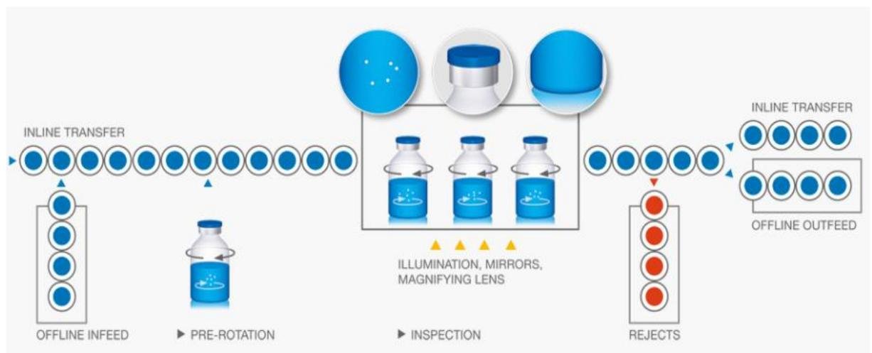
SCHEMATIC REPRESENTATION OF SEMI-AUTOMATED INSPECTION PROCESS
